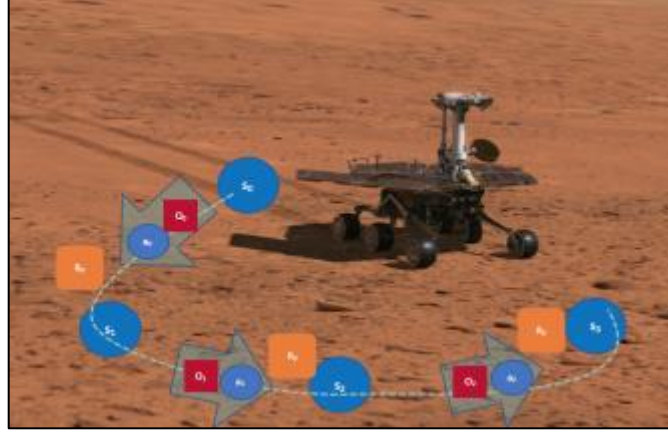
Figure 4: A partially observable Markov decision process representation with 3 states ( s_0, s_1, s_2, s_3 ), and 3 corresponding observations ( o_0, o_1, o_2, o_3 ), actions ( a_0, a_1, a_2, a_3 ), and rewards ( R_0, R_1, R_2, R_3 ) respectively.
